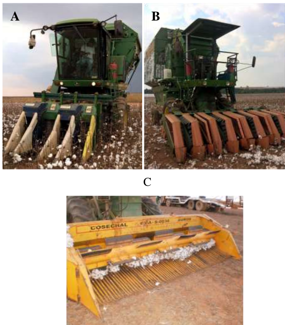
Figure 1. (A) John Deere picker harvesting with platform type Pro-12 VRS, (B) Harvester with brush-type picking platform with a view of the coupled field cleaner used in both experiments, (C) Harvester with finger type harvesting platform.
